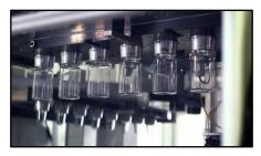
Use ISBM to manufacture bottles that have small to medium bodies and relatively small necks. We use ISBM to manufacture all of our Polyethylene Terephthalate (PET) bottles.
