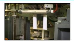
Use the EBM process to manufacture large-size, High Density Polyethylene (HDPE), Low Density Polyethylene (LDPE), and Polypropylene (PP) bottles with large necks.
